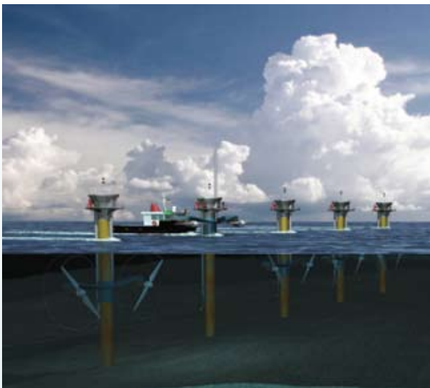
▼ A conception of a field of water mills designed by Marine Current Turbines that turn the currents of tides into electricity.
